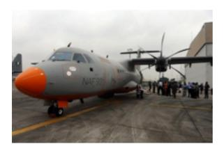
It includes sensors, radar and Electro-Optic Surveillance and Tracking (EOST) equipment, which houses three cameras to monitor ships in Nigerian waters, said Sergeant Sunday Olalekan Omotosho.
